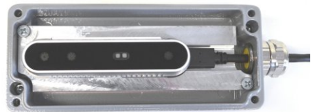
The mount guarantees good heat dissipation
