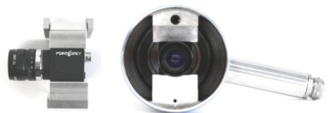
The mount guarantees good heat dissipation
