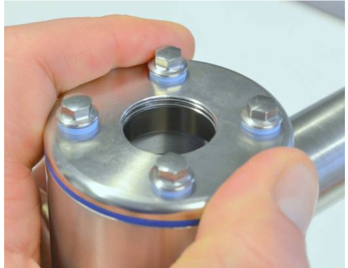
Mount rear wall after mounting the camera inside the enclosure! Feed cables through the rear wall fist! Hold rear wall down firmly in order to avoid gaps (see below). Rotation might assist proper assembly. The “push-locking” assembly makes it a lot easier to assemble/ remove the rear lid compared with screw-mounting – especially with cables attached to the camera!
