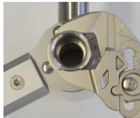
Tighten Adapter and cable gland body, which can also be mounted with Loctite 577 as a precaution.
