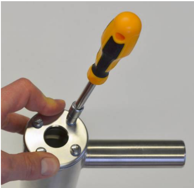
Tighten the hygienic screws cross-wise while holding the lid down.
