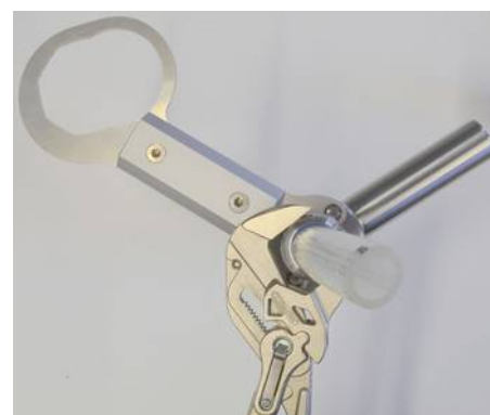
Hold rear lid again with the mounting tool and tighten the cable gland cover nut.
