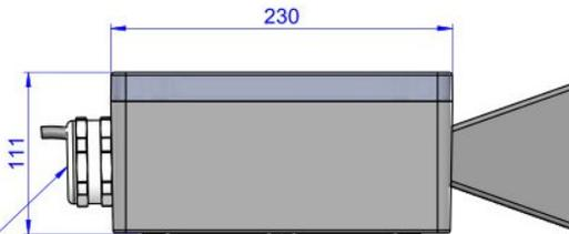
M50 cable gland for large connectors that fit through 42mm diameter aperture
