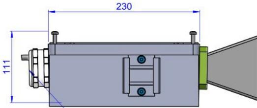
M50 cable gland for large connectors that fit through 42mm diameter aperture
