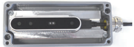
The mount guarantees good heat dissipation
