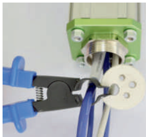
The Spreading Pliers are helpful to insert cables into the cable gland insert
