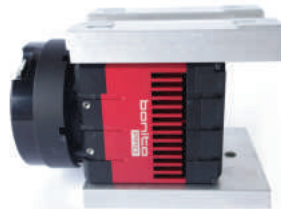
The mount guarantees excellent heat dissipation
