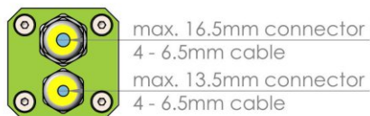
Rear Wall B
